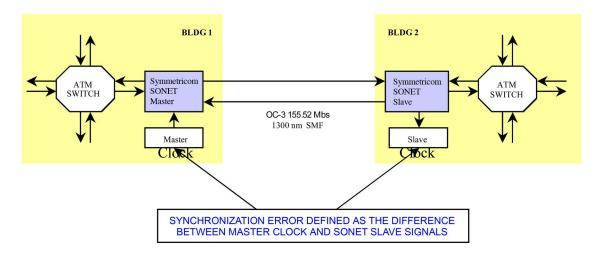
FIG.4 Typical Time-Based Communications Implementation
