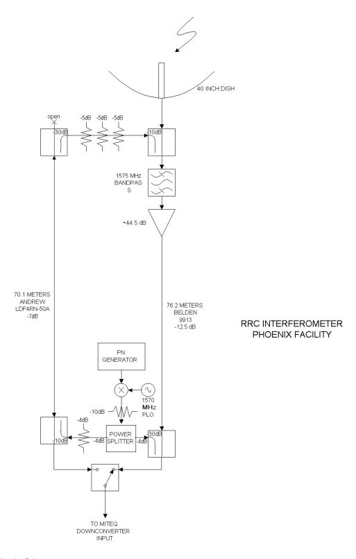
FIG.3 L-Band RF and Calibration Subsystem
