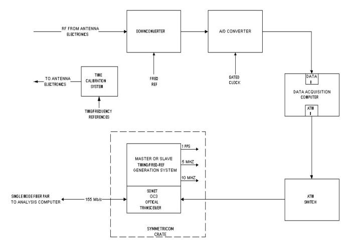
FIG.2 Diagram of CEI Equipment at Each Site
